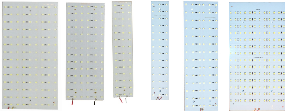
126 LED SMD PCB 84 LED SMD PCB 42 LED SMD PCB 42 LED PCB METAL 84 LED PCB METAL 168 LED PCB METAL
